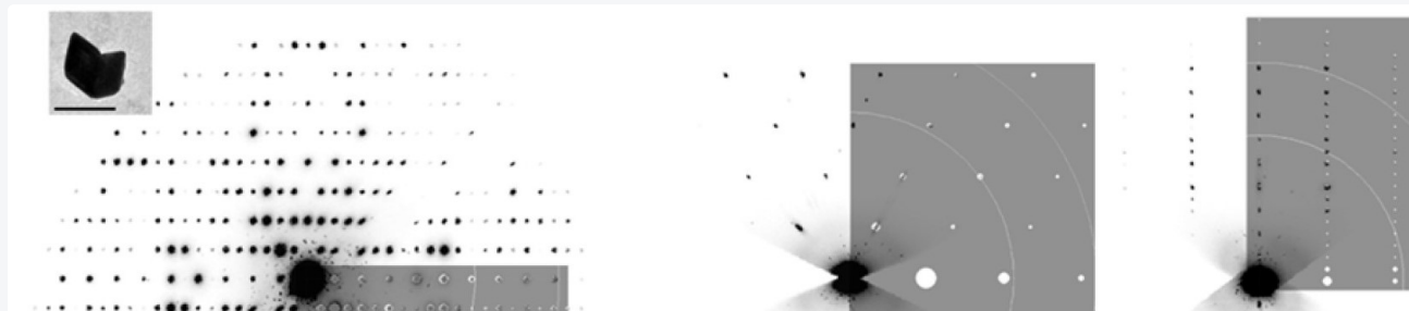
Fig. 2 With the ELDICO ED-1, the experimental diffraction data (left) show a perfect match with the simulated data (right).
